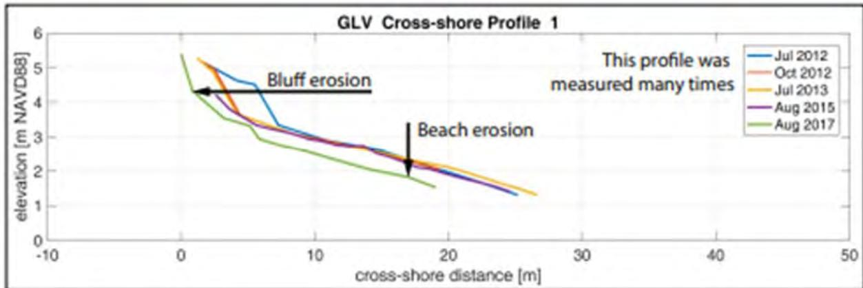
*This beach at Golovin has been measured five times over five years. The x-axis is the horizontal distance from the bluff to the water. The y-axis is the height of the ground along this profile. The repeated profile measurements tell us how the beach is changing; the bluff eroded about 5 meters over the time period, but the beach was stable for three years and then eroded about 50 cm in two years.*
