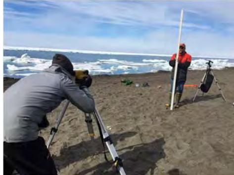
This method requires a sighting level. Hand-held sighting levels work fairly well but borrow more precise equipment (surveyor's level on a tripod or laser level) if possible.
