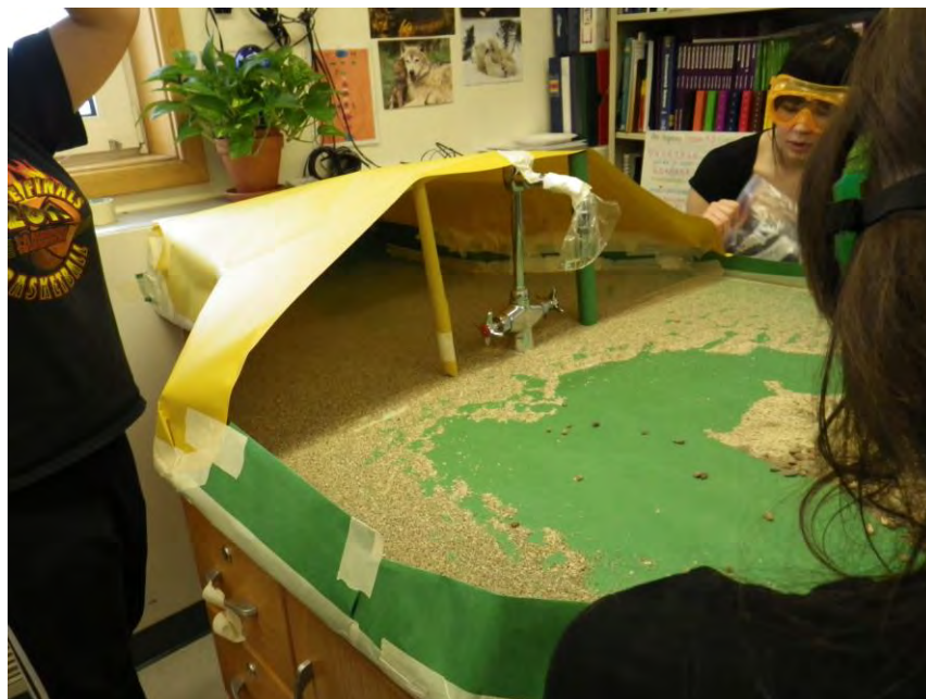
Set-up for wind erosion experiment. Sand has already been blown by the wind.
